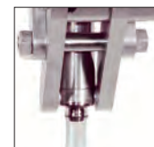
Spent primers collected and dropped into a flexible plastic tube for easy emptying.
